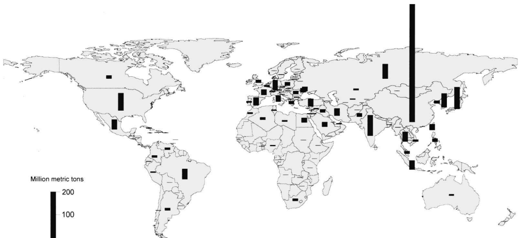
Figure 2 World distribution of annual cement industry CO 2 emissions potential based on country clinker capacities in the mid-1990s. By far, the greatest emissions potential is in Asia. Source: Based on data in Cembureau (1996).
